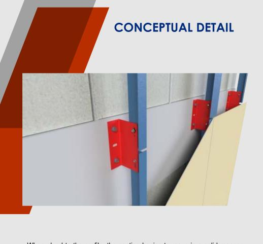
When glued to the profile, the coating begins to move in a solid manner. Therefore, it must strictly respect the division between panels, with expansion joints being indispensable and unquestionable. It is precisely at this point that the greatest deviations occur, due to the practical difficulty of execution.
