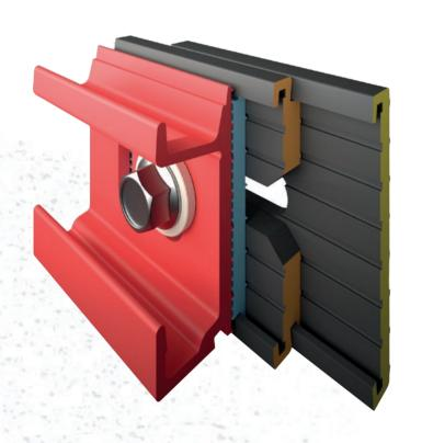
The shims are available in different thicknesses, allowing planimetry adjustments of up to 2 centimeters and regulations of 2 in 2 millimeters. The use of these wedges is simple and their objective is to correct small deviations in the planimetry of the existing façade.
