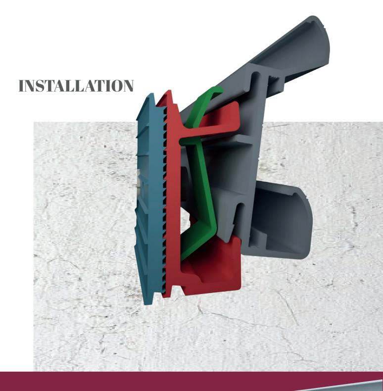
The union of the horizontal profile with the CLAW support, due to its peculiar design, allows expansion movements, because the fixation is carried out with clips and not with screws that block the movement. This mobility allows the profile to accommodate changes in temperature and shrinkage of the building without causing stress or structural damage.
